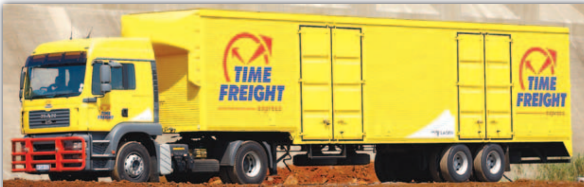
Time Freight, a national express road freight business with headquarters in Pietermaritzburg, uses 6x4 Man line-haul units that are rated for 480 hp but only operate with a payload around 24 tons to maintain high average speeds.
